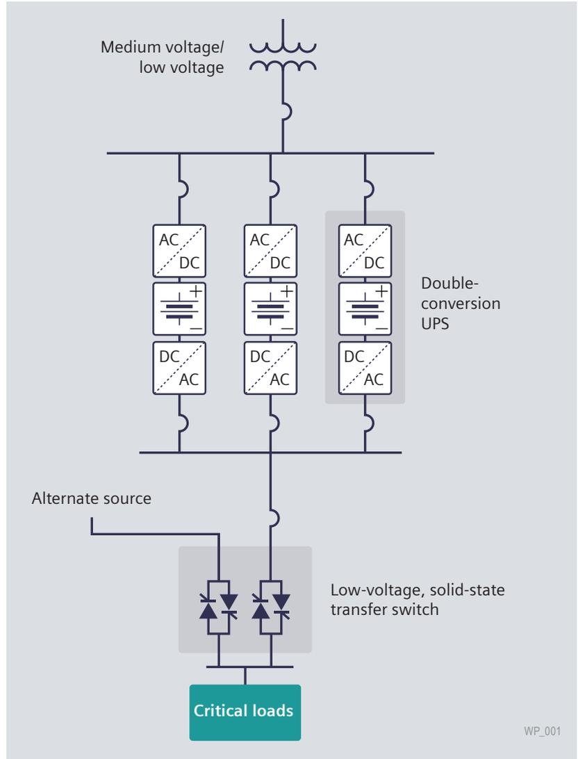
Figure 1: Typical system with double-conversion LV UPS
