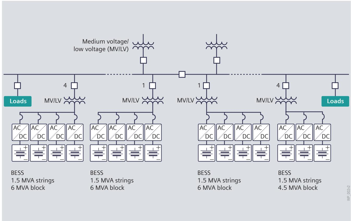
Figure 2: Typical medium-voltage system with BESS system at medium voltage. Each BESS block can be made of up to four 1.5 MVA strings. BESS blocks can be added as needed.
