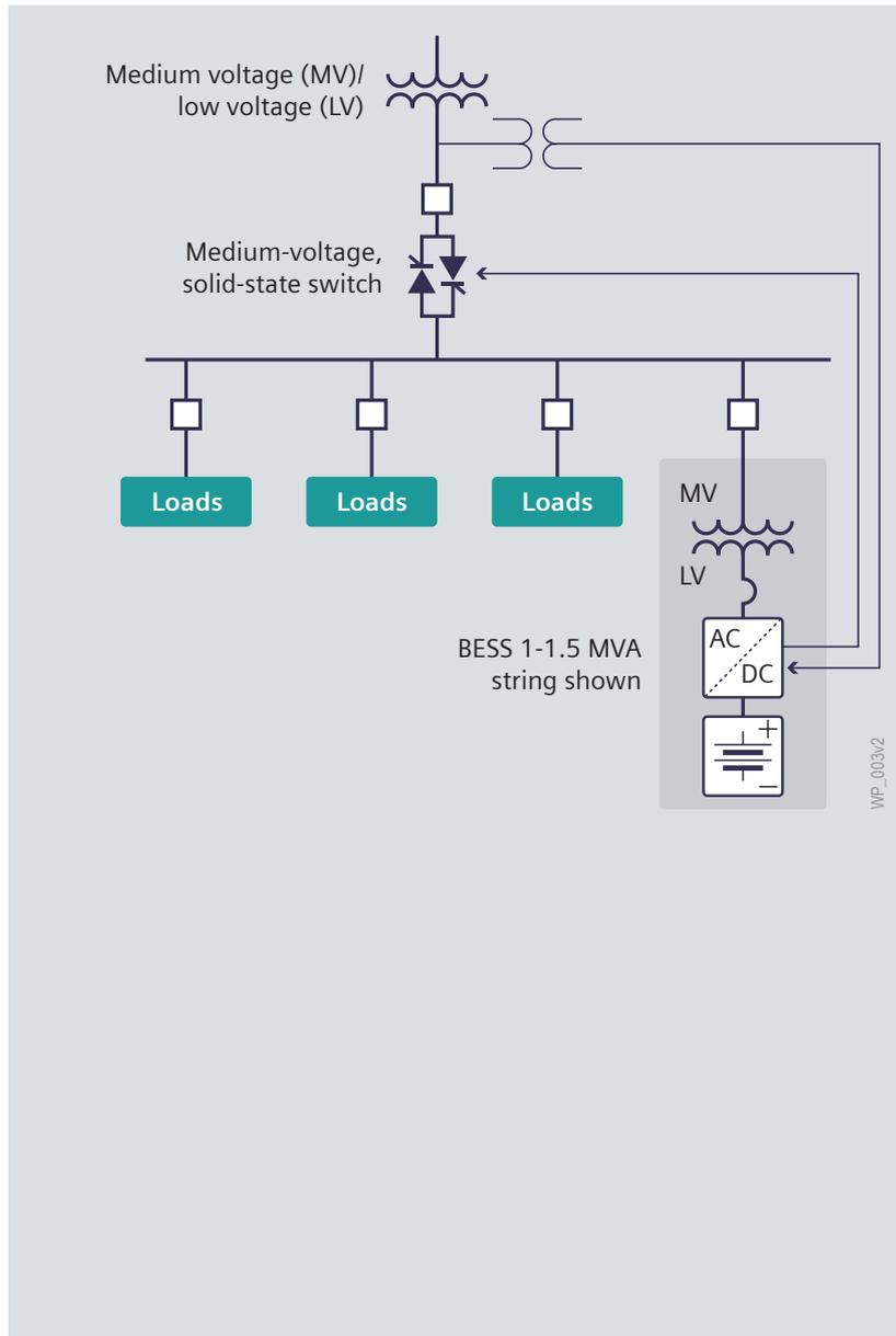
Figure 3: Typical BESS system with MV solid-state switch and direct voltage connection to inverter at the BESS system to be able to achieve between 12 ms-15 ms of transfer time.
