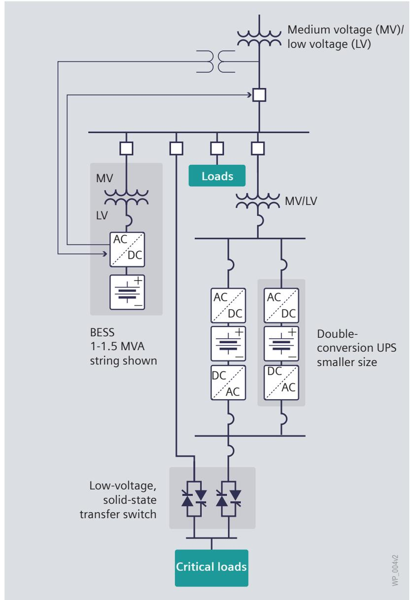
Figure 4: Hybrid scheme integrating MV BESS and reduced-in-size LV UPS. MV solid-static switches are not required.
