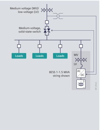
Figure 3: Typical BESS system with MV solid-state switch and direct voltage connection to inverter at the BESS system to be able to achieve betweem 12 ms-15 ms of transfer time.
