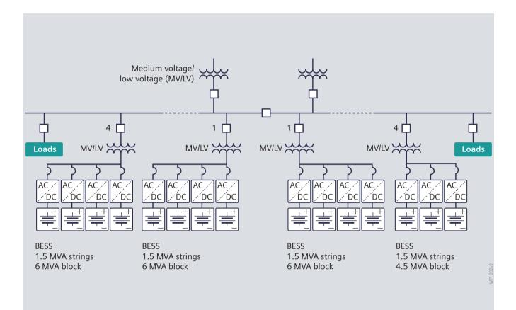
Figure 2: Typical medium-voltage system with BESS system at medium voltage. Each BESS block can be made of up to four 1.5 MVA strings. BESS blocks can be added as needed.
